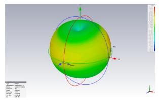
Fig. 4 Directivity of antenna @ 5.54 GHz in CST 2016.
