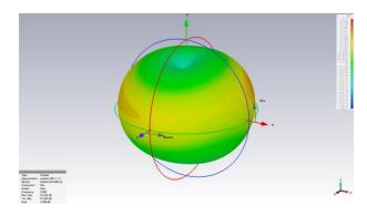
Fig. 3 Gain of antenna @ 5.54 GHz in CST 2016.
