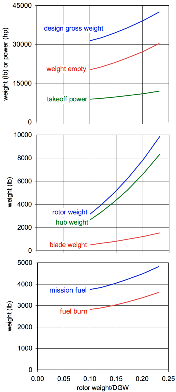
Figure 38. Influence of rotor weight technology (rotor weight fraction of design gross weight) on civil aircraft with scaled rotor weight model.
