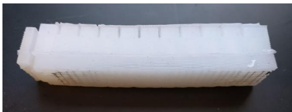
Figure 2. Hybrid soft bending actuator design with inlaid mesh tape.
