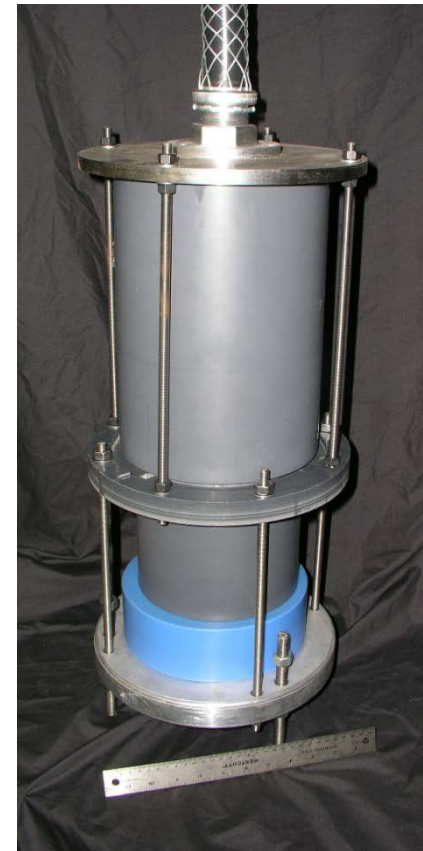
Fully assembled blue nylon base HV feedthrough
