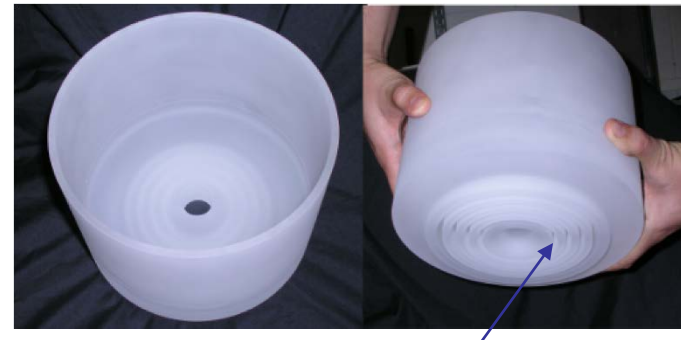
Grooves increase path length to ground
