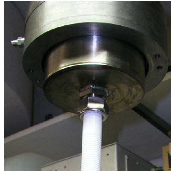
Swagelok style oil to vacuum seal
