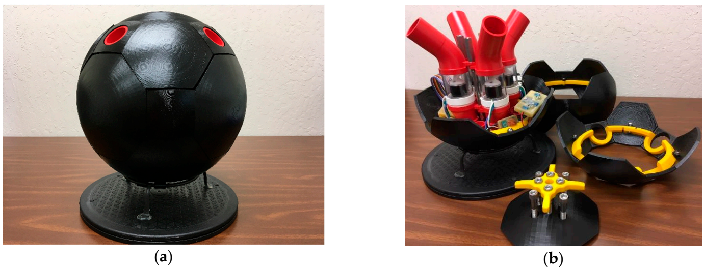
Figure 1. The Wreck Interior Exploration Vehicle (WIEVLE). (a) WIEVLE, on its test stand; (b) Plated hull removed to reveal WIEVLE's propulsion system.
