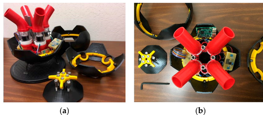
Figure 13. Propulsion core (a) Oblique (b) Top-down view. Note the four lower retention bolts capped by coupling nuts, which will join with the four upper bolts. Batteries and buoyancy foam are removed.
