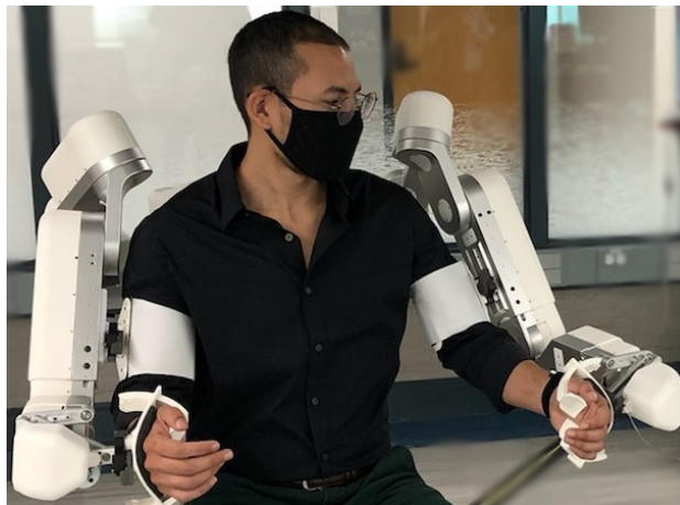
Fig. 1: The Eminence Grip facilitates consistent and stable connection between the human and the Harmony Exoskeleton by constraining the hand in a comfortable and adjustable novel interface.
