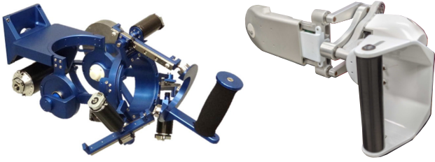
Fig. 2: The typical handle design, as seen in the MAHI Exo [14] (left) and the Harmony Exoskeleton [15] (right), require active interaction from the user and can create undesirable sensory and biomechanical couplings between the hand and the proximal joints of the upper extremity.
