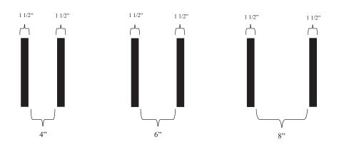
Contrast striping, 4-inch with 1-1/2 inch black border Contrast striping, 6-inch with 1-1/2 inch black border Contrast striping, 8-inch with 1-1/2 inch black border
