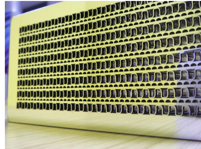
Fig. 6, section through a H 2 X (counter-flow).
