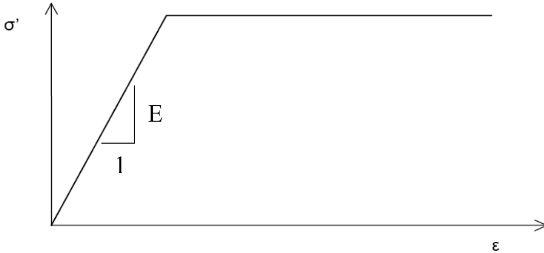
Figure 3.7: Stress-strain relationship for the Mohr-Coulomb model (Plaxis, 2005)
