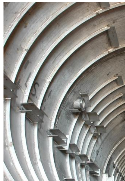
Figure 3: Tray internal Support Rings (Photo Courtesy Dacro Industries)
