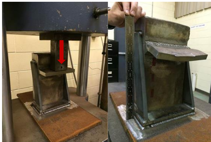
Figure 8 a) Test Article in Test Frame and b) After Application of 534kN: Cantilever Testing of Direct Attachment Welded to Explosion Clad Material
