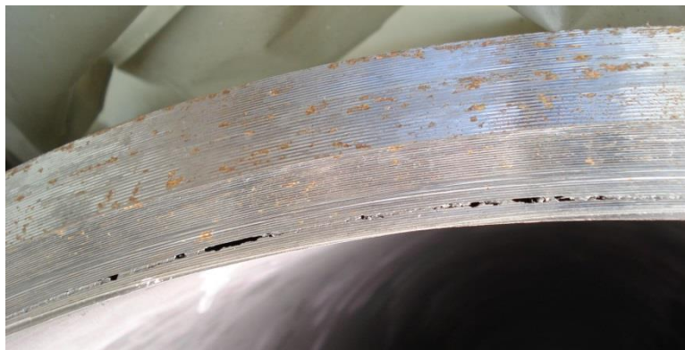
Figure 13: Hot Roll Bond, Disbonding after Forming
