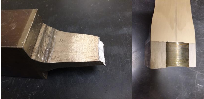
Figure 11: Examination of Simulated Non-Bond Test Specimen – No Clad Separation
