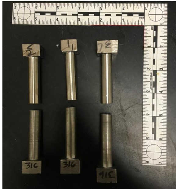
Figure 14: Roll Bond Samples with Brittle Failure in the Bond Zone
