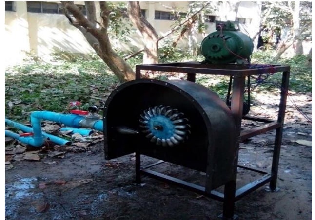
Figure 11. Assembly of Pelton Turbine
