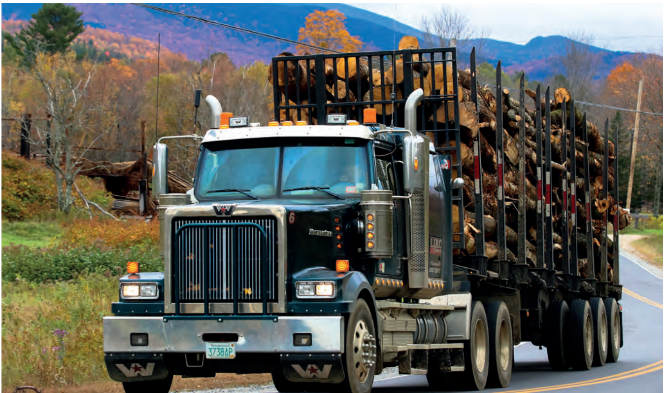
Logging trucks are a common heavily laden, multi-axle truck that can increase pavement loading dramatically. (Photo courtesy Mussi Katz)
