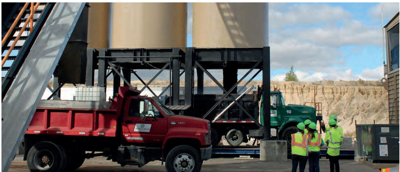
Using multiple drops from the silo to load a haul truck can help to avoid truckload-to-truckload segregation.
