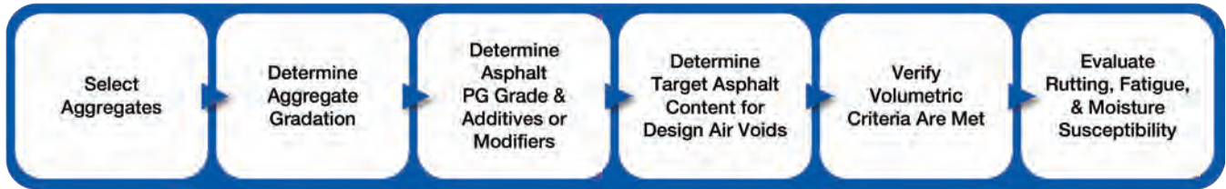
Figure 6-1. Flow Chart of Asphalt Mixture Design
