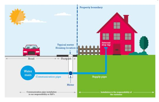
The supply pipe shall be the property owner's responsibility and shall conform to the Water Regulations and requirements of the Water Company.
