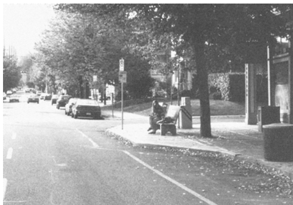
FIGURE 7-9 BUS STOP WITH CURB EXTENSION
