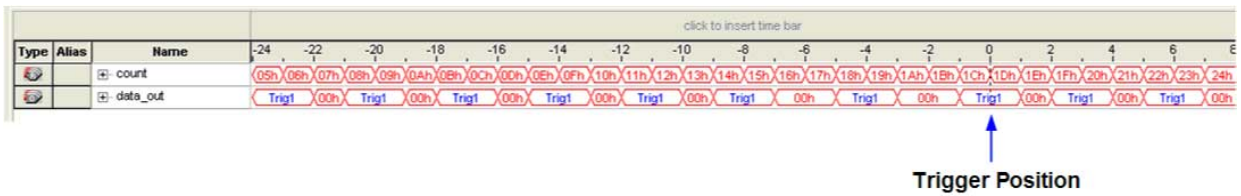
Figure 13-50: SignalTap II Logic Analyzer Continuous Data Capture
