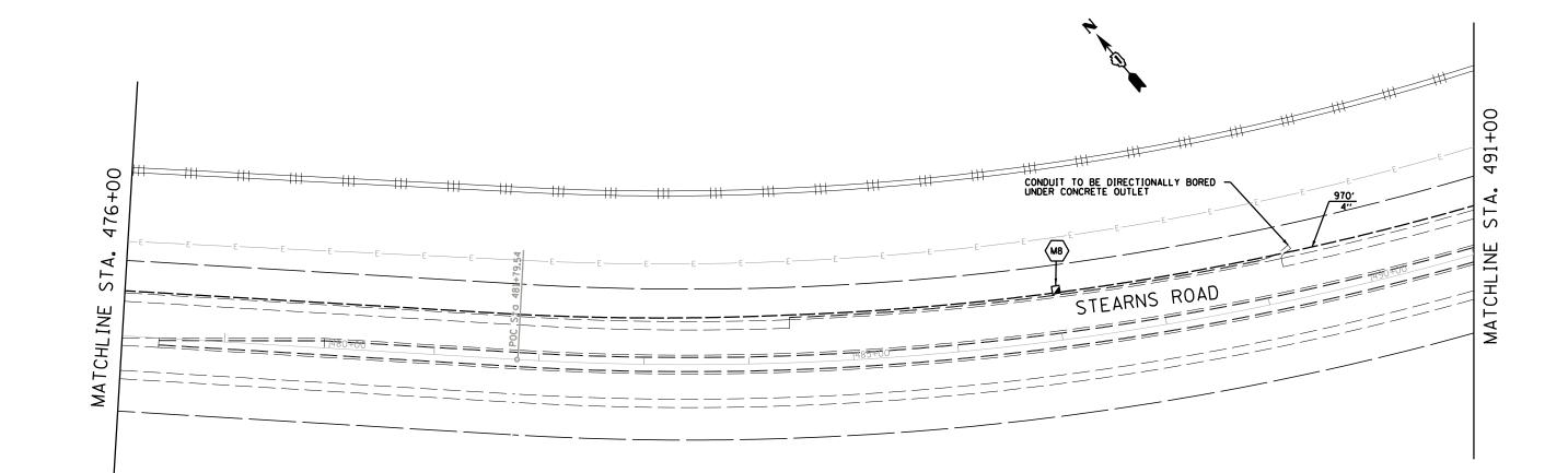
1. UNDERGROUND CONDUIT FOR FIBER OPTIC BACKBONE SHALL BE INSTALLED 2' BEHIND BACK OF CURB OR BACK OF SHOULDER UNLESS OTHERWISE INDICATED ON THE PLANS.
