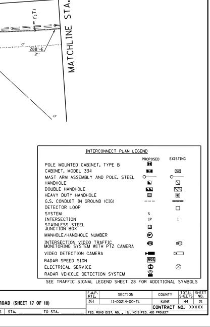
EXISTING CONDITIONS SHOWN REPRESENT THE PROPOSED ROADWAY CONFIGURATION BEING CONSTRUCTED UNDER IDOT N CONTRACT NO. 63598. CONTRACTOR MUST VERIFY ACTUAL CONDITIONS PRIOR TO COMMENCING WORK IN THIS SECTION OF STEARNS ROAD.
