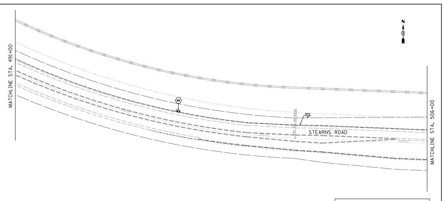
1. UNDERGROUND CONDUIT FOR FIBER OPTIC BACKBONE SHALL BE INSTALLED 2' BEHIND BACK OF CURB OR BACK OF SHOULDER UNLESS OTHERWISE INDICATED ON THE PLANS.
