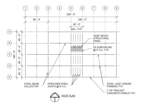
Figure 2-2. Example's roof plan
