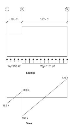
Figure 2-5. North-south diaphragm loading
