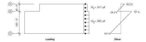
Figure 2-4. East-west diaphragm loading
