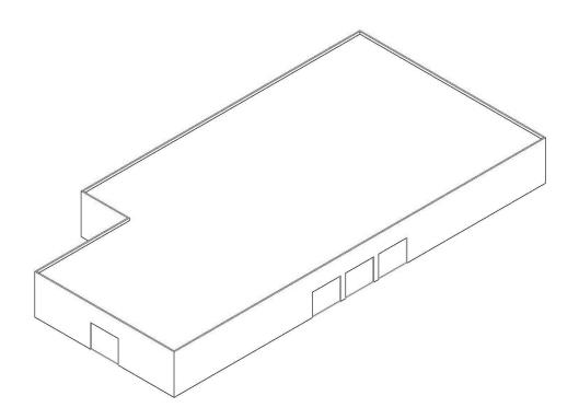
Figure 2-1. Typical building with flexible diaphragm
