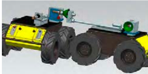
Two UGVs connected by the coupling and actuating system
