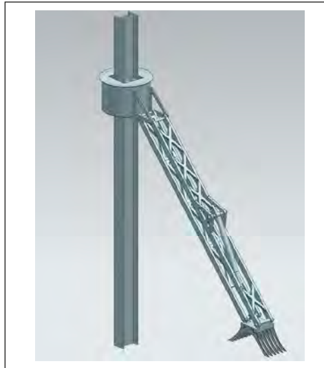
Solid model geometry of proposed effector
