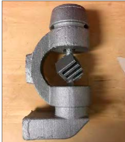
3D-printed pattern cast in aluminum by Mercury Marine
