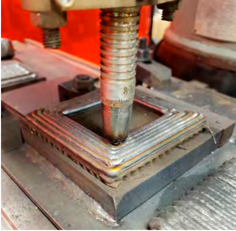
WAAM construction of a coupler for the die casting process
