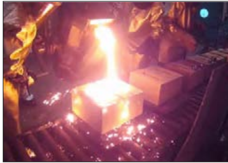
Pouring SSFDI into one-inch Y-blocks in the Michigan Tech Foundry
