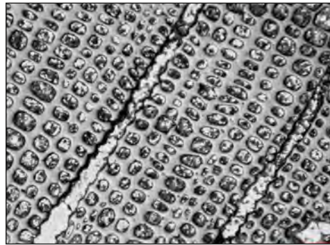
Carbonized wood pores infiltrated with magnesium metal
