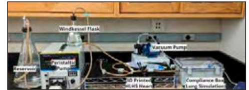
Benchtop design simulates physiological conditions in HLHS patients for testing of our stent prototype
