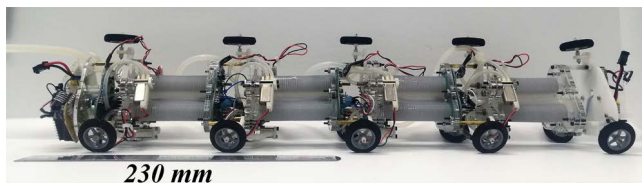
Fig. 1. The 3-D Soft Snake Robot. The body length of the SRS is 530 mm, and the height is 100 mm. The length of each module is 100mm, which is made up of 70 mm of bending segment and connectors.
