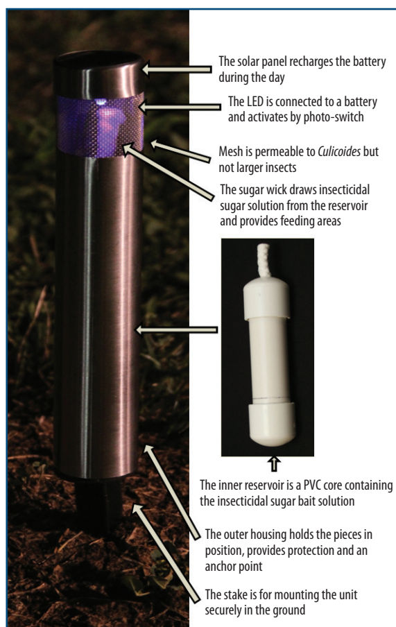
Figure 1. Insecticidal sugar trap. The bait station is a modified lawn light equipped with an ultraviolet light emitting diode (LED) and an insecticidal sugar bait.
