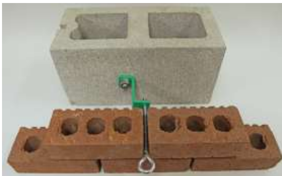
Figure 1 This photo shows how building ties can be designed so that they are easier to remove and can be reused.
