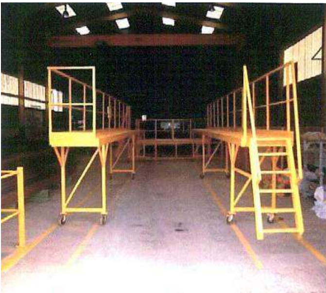
The above two photos show how movable platforms with guardrails can be used around the open sides of a truck bed when loading and unloading trucks
