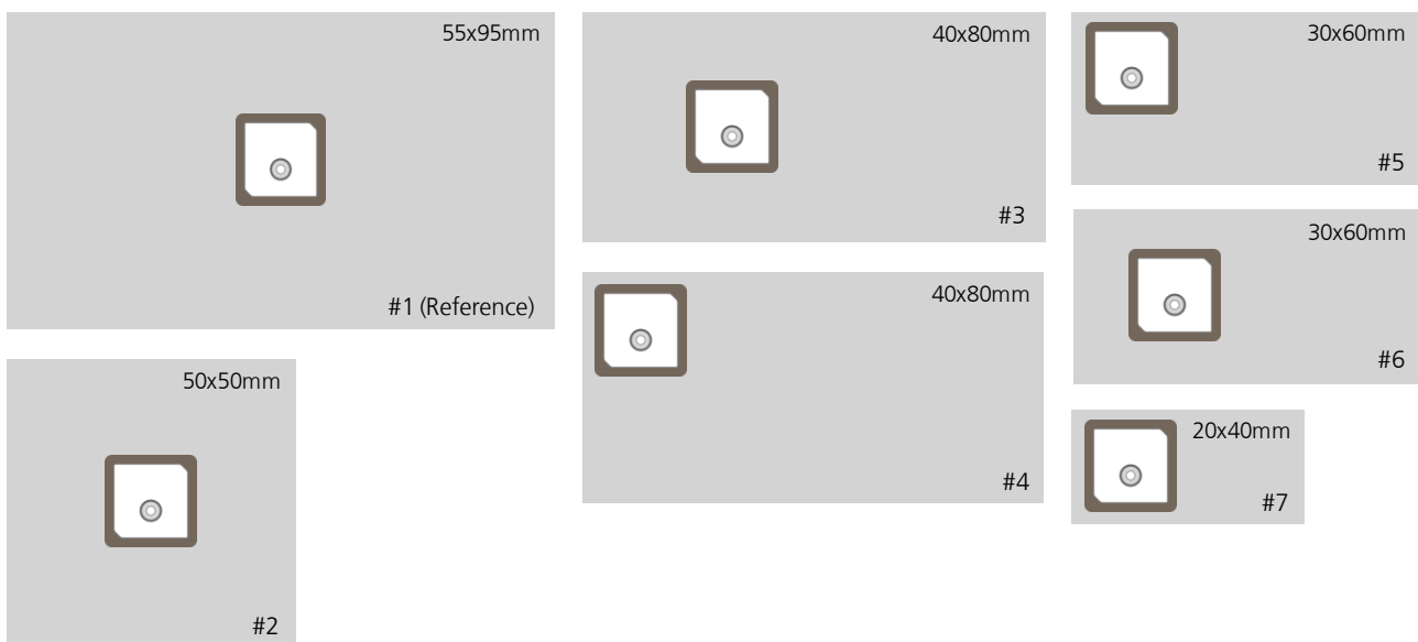
Figure 9: SAM-M8Q on different GND planes
