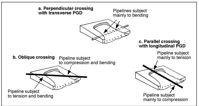
Figure 1. Direction of Permanent Ground Deformation (PGD)
