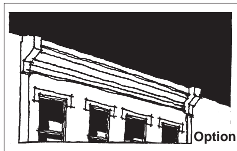
A simplified version of the original, using the major lines of the original, may be considered.
