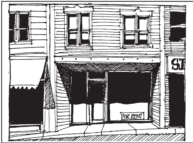
Inappropriate storefront replacement.
