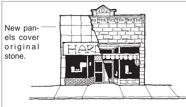
Covering original materials is inappropriate.
