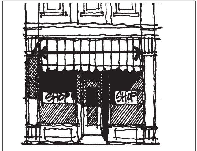
This awning fits within the width of the existing opening.
