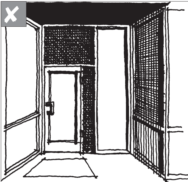
Don't close down the opening to make a smaller door fit.
