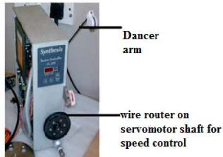
Fig. 8 : Final device with controller card and peripherals assembled.
