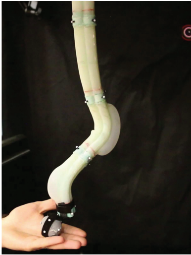
Fig. 1. Soft fluidic elastomer manipulator gently taking a small ball from the palm of its human collaborator. The manipulator's entirely soft composition and kinematic controller allow it to safely interact with its environment. Reproduced with kind permission from Mary Ann Liebert Inc. (Marchese et al., 2015a).
