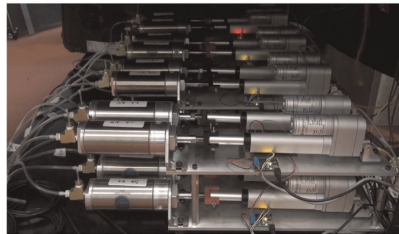
Fig. 15. Top: schematic representation of a high capacity fluidic drive cylinder. The device consists of a (a) fluidic cylinder, (b) piston, (c) linear drive, and (d) electric motor. Bottom: An array of 16 fluidic drive cylinders used to power the spatial soft arm. Reproduced with kind permission from the IEEE (Marchese et al., 2015b)
