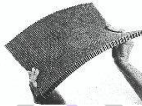
Figure 5 : Anticlastic curvature of core
