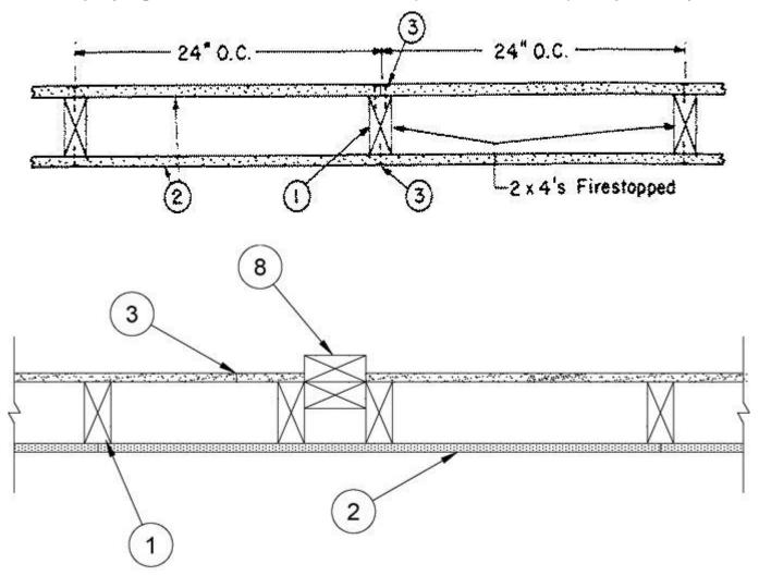
1. Wood Studs — Nom 2 by 4 in., spaced 24 in. OC effectively firestopped.
