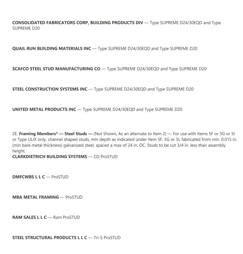
2F. **Framing Members\*** — **Steel Studs** — Not Shown — In lieu of Item 2 — proprietary channel shaped steel studs, minimum width indicated under Item 5, 1-1/4 in. deep fabricated from min 0.015 in. (min bare metal thickness) galvanized steel. Studs 3/8 in. to 3/4 in. less in lengths than assembly heights. **SUPER STUD BUILDING PRODUCTS** — The Edge
