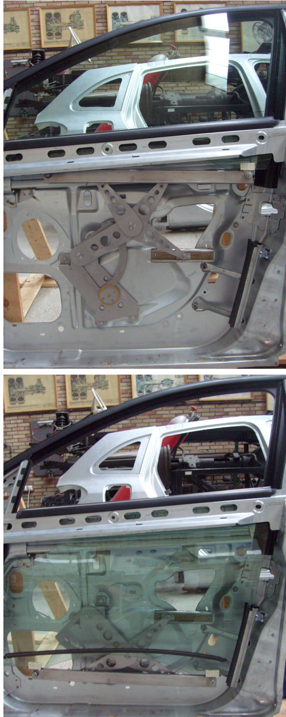
Figure 4.9 Assembled window regulator prototype on the car door chassis at the top and lowest positions
