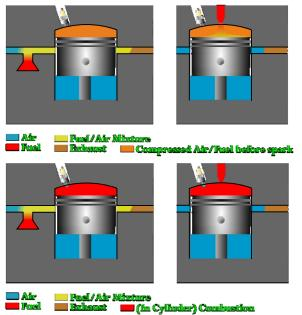
Figure 1 Carbureted vs. Direct Injected Two-Stoke Operation
