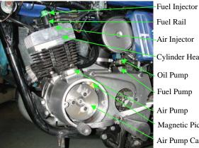
Fuel Rail Air Injector Cylinder Head Oil Pump Fuel Pump Air Pump Magnetic Pick Up Air Pump Cam
