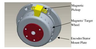
Figure 4: Replacement Magneto with 24 Minus 1 Tooth Count and Magnetic Pickup
