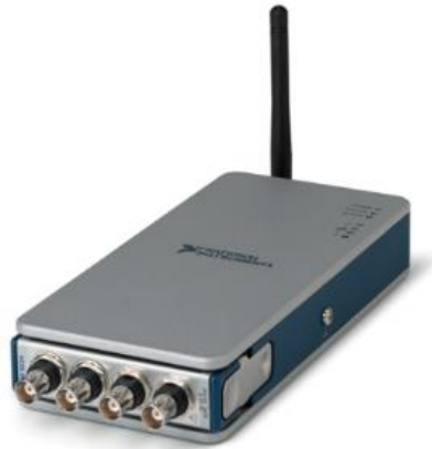
Figure 9: National Instruments Wireless DAQ Box (National Instruments Corporation)
