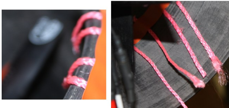
Figure 3.11. Flow visualization - the flow field appears attached throughout the shroud. Left: The prototype shroud inlet with tufts attached. Right: The same shroud, with tufts attached to the rear at the diffuser. Separation does not appear to be an issue.
