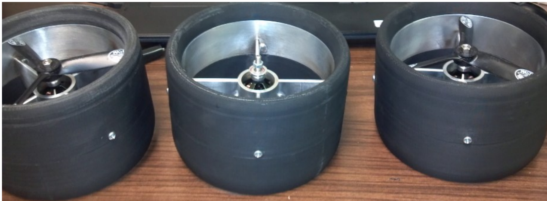
Figure 3.17. The three assembled shrouds used on the final assembly of the vehicle.
