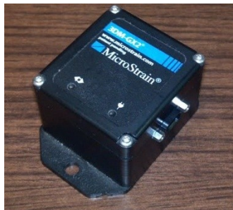
Figure 5.1. A picture of the MicoStrain 3DM-GX2 IMU. This unit will be mounted onboard the supply vehicle to gather the dynamic states of the vehicle.
