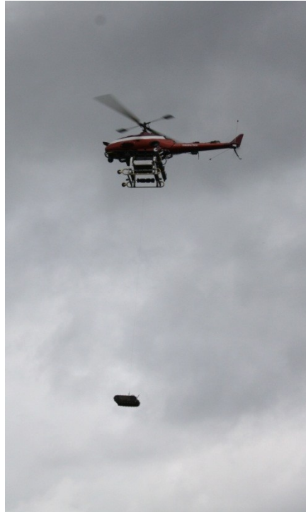
Figure 2.1. A ground robot being deployed from the VT Unmanned System Lab Yamaha R-MAX.
