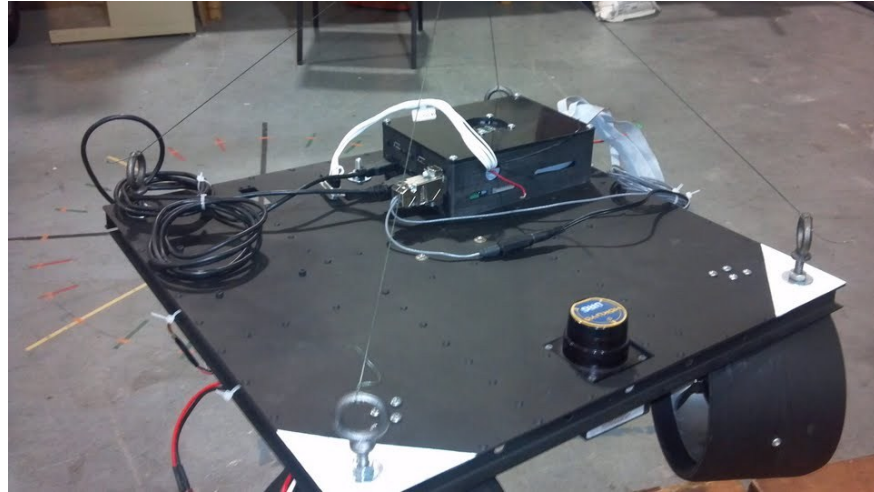
Figure 5.15. The vehicle with all of the subsystems installed. Note that the corners were painted white in case cameras were to be used to collect orientation and position information.
