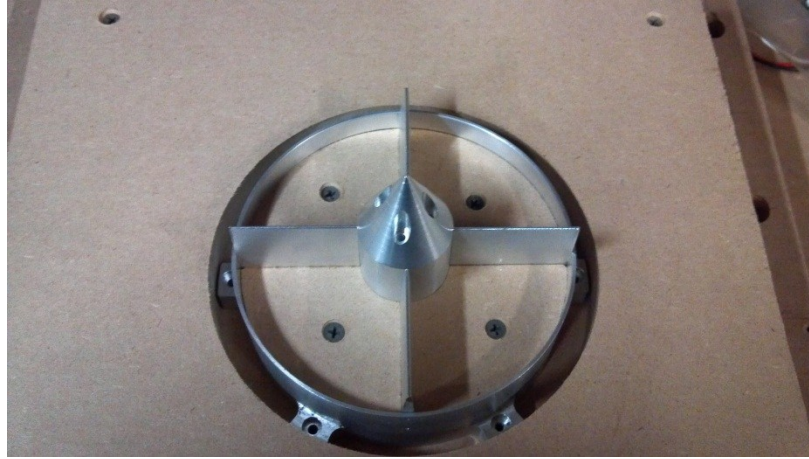
Figure 3.16. Shroud center assembly fixture, used to place the components in their proper plane and to ensure that they were concentric.
