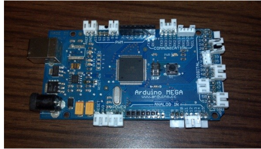
Figure 5.3. A picture of the Arduino MEGA. The Arduino MEGA was selected to provide a pulse width modulated signal to the electronic speed controllers.
