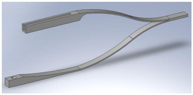
Figure 12.5. CAD drawing of forceps without sliding mechanism
