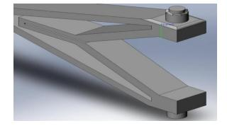
Figure 12.7. Interface featuring inclined cylinder that would function like a ratchet to allow lateral rotation.
