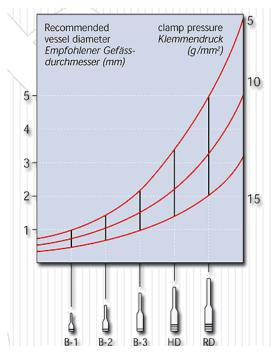
Figure 12.1. Recommended clamps for certain vessel diameters and required clamping pressure (S&T 2007)
