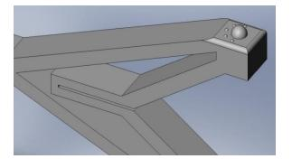
Figure 12.8 A large half-sphere allowing vertical rotation with smaller half-spheres surrounding it to allow the clip to be locked into different lateral angles.
