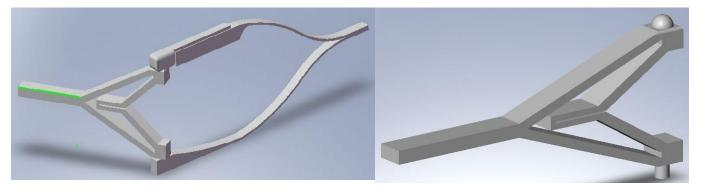
Figure 4.1. Preliminary design featuring spherical and cylindrical clip interfaces (right) and a sliding mechanism on the forceps (left).
