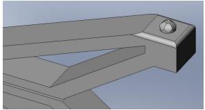
Figure 12.9. Hexagonal half-sphere that would function as a ball-end hex key to lock the clampinto different angles.
