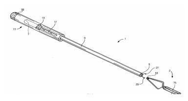
Figure 2.6. Schematic of hook bulldog clamp applicator (Stevens and Rapacki 1996)
