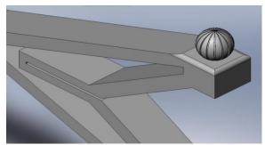
Figure 12.10. A spherical interface with slotted grooves allowing both lateral and vertical rotation, locking the clip into place.
