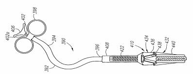
Figure 2.7. Schematic of flexible clamp applicator (Glines, Morejohn and Septeka 2000)
