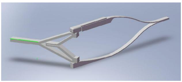
Figure 12.3. This image depicts the full assembly of the initial forceps, sliding mechanism, and clamp design.
