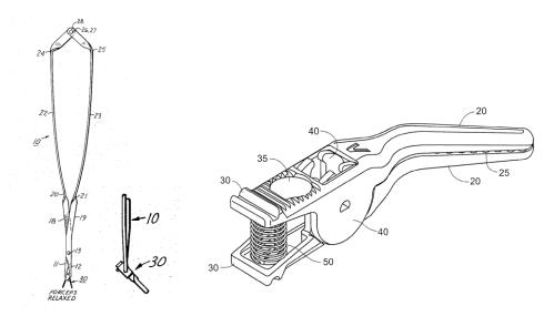
Figure 2.4. a) Schematic of a new spring-loaded forceps that incorporates a pivoting arm (left) (Cogley 1974) and b) a clip with angled jaws (right) (Kuester 2006)
