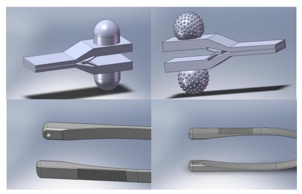
Figure 4.2. CAD drawings showing the smooth spherical interface on the clip (top left), the spherical interface with surface irregularities (top right), and the spherical inverse (bottom left) and track (bottom right) interfaces on the forceps.
