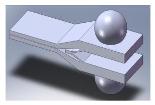
Figure 12.11. Smooth spherical interfaces that would allow unlimited vertical and lateral rotation based on friction.
