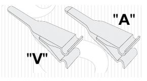
Figure 12.2. Variations in clamp shape to accommodate for different vessel sizes and pressures (S&T 2007)
