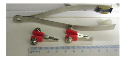
Figure 5.1. Forceps with cap and track interfaces (top), clip with spherical interface with surface irregularities (bottom left), and clip with smooth spherical interface (bottom right).
