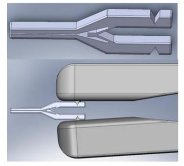
Figure 2.3. Diagram depicting the groove interface of the currently used clips (top) and the tongue-and-groove interface of the currently used microvascular clip-forceps system (bottom).
