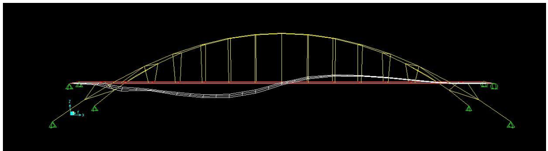
Figure 47. Influence line for torsion force for 2nd arch member in from start of span.
