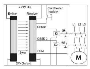
Fig. 3. Through beam switching system connection to the motor
