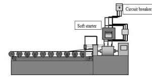
Fig. 5. Belt and power saving system
