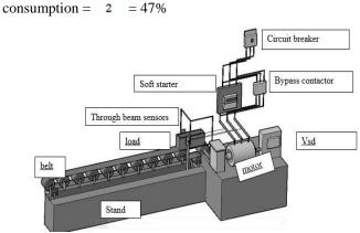
Fig. 4 Auto CAD diagram layout.
