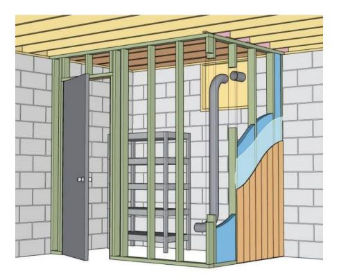
*Figure 8: Basic ventilation system in a cold cellar (Trandem, 2013)*
