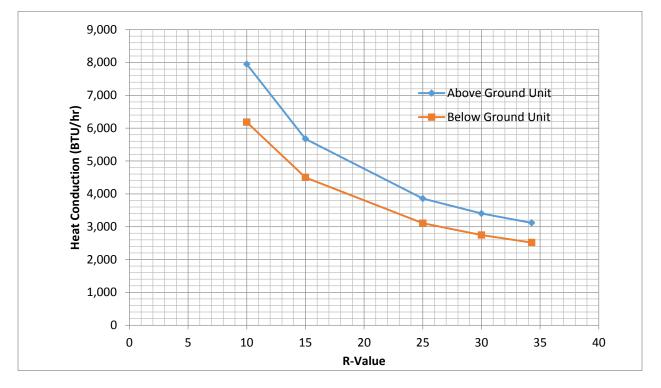
Figure 23: R-value vs. Heat conduction trend in the above ground and below ground units
