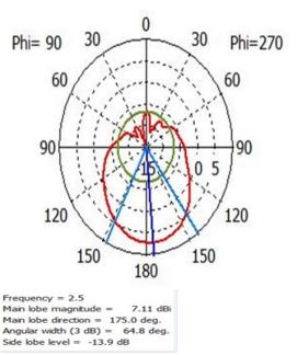
Fig.5. Far field of 7.11 dB at the centre frequency of 2.5 GHz.
