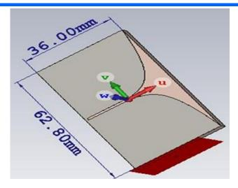
Fig.1. Top view of the proposed antenna.
