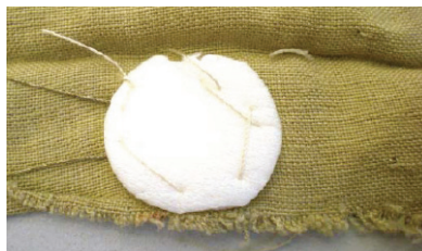
Figure 16. The temperature sensor isolated by cotton foam.
