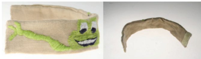
Figure 15. The prototype belt for monitoring body temperature.
