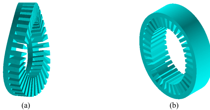
Fig. 4.1. (a) Mode shape for an axial-flux machine stator at the frequency of 497 Hz. (b) Mode shape for the radial-flux machine stator at the frequency of 355 Hz. Parameters used in both cases: D_o = 328 mm, Q = 36 , y = 40 mm, l_y = 19 mm. Structural damping due to the lamination is not included in the computation model.
