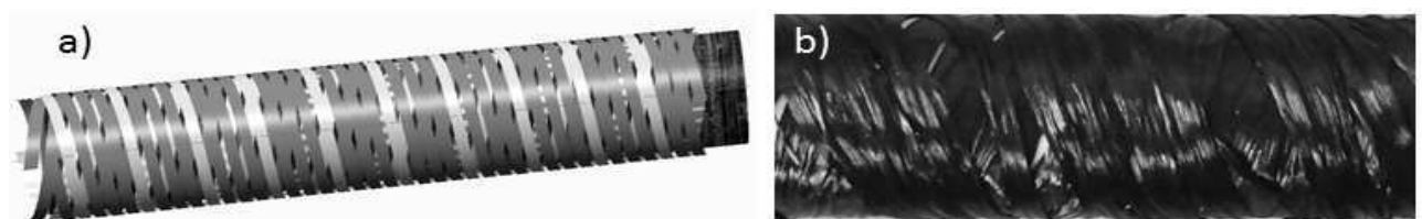
Fig. 2 The wound tube a) CAD model b) Real part
