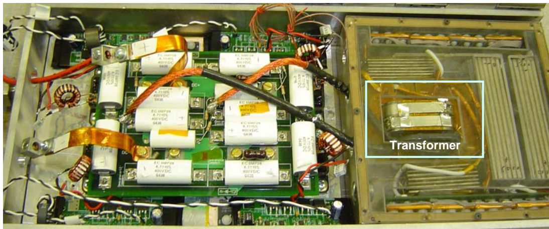
Fig. 5-16 30 kW PRC system with the nanocrystalline transformer
