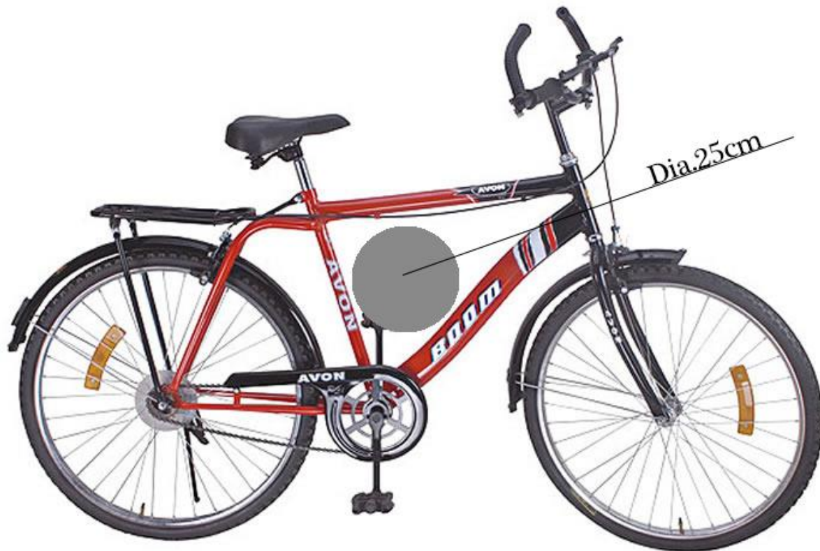
Fig.6.1 position of flywheel in a bicycle [30]
