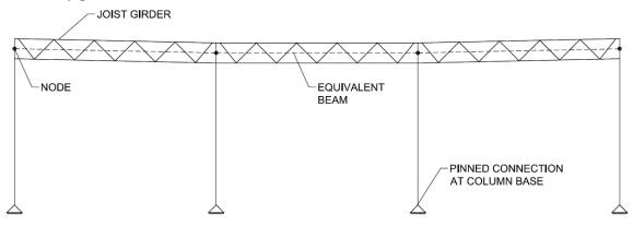
FIGURE 1 SIMPLIFIED STRUCTURAL MODEL 1
