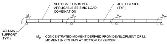
FIGURE 3 STRUCTURAL MODEL 2
