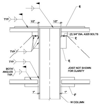
FIGURE 4 MOMENT CONNECTION TO AN INTERIOR COLUMN
