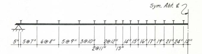
The design resulted in the use of 32 sets of 3- $\frac{7}{8}\phi$  studs per half of the beam or a total of 192 studs. Theoretically, the number of studs may be determined as follows:
