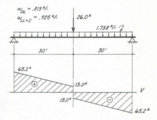
To determine the spacing of the studs, the theoretical spacing is calculated at, say, 5 foot intervals along the span and a theoretical curve plotted to scale. From this curve the actual spacing is determined with the AASHO limitations of a 6" minimum and a 24" maximum spacing. The following spacing was adopted:
