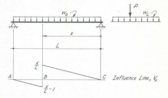
The portion of the span BC would be loaded with the movable uniform load and the concentrated load, P, would be placed at B to produce the maximum shear at the point B. Therefore, due to live load,
