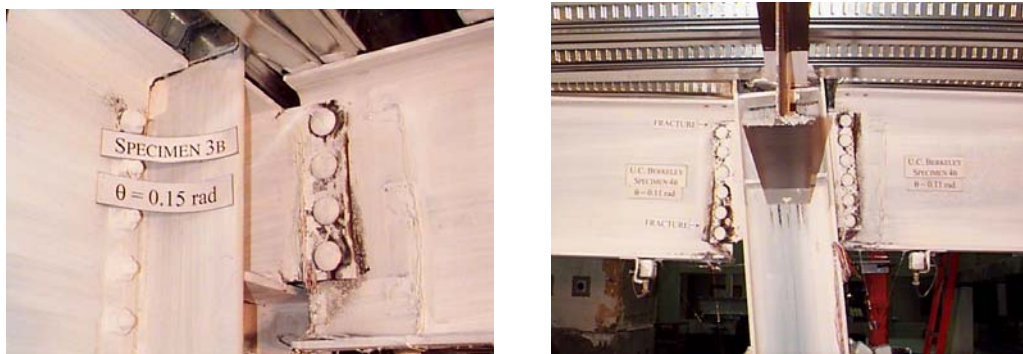
Figure 3.3. Fracture of Net Area under Very Large Rotations (Larger Than 0.09 Radians)
