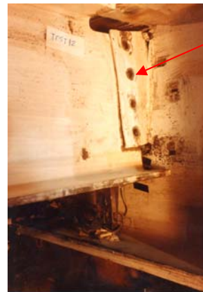
Figure 2.19. Failure of Specimen 12, a Beam-to-Girder Shear Tab Connection
