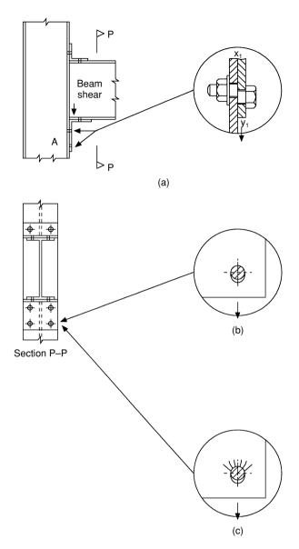
**Fig. 4.52** Failure modes of a beam-to-column connection: (a) single shear failure of bolt; (b) bearing failure of bolt; (c) bearing failure of cleat.
