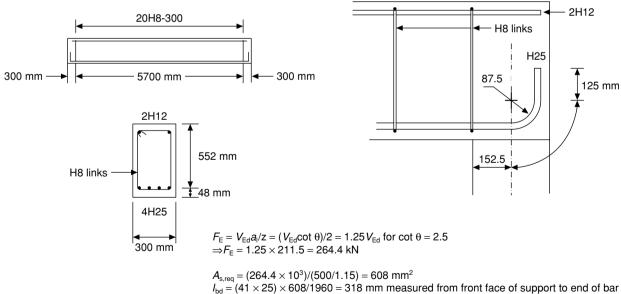
$\geq 0.3I_{bd,reg} = 0.3 \times (41 \times 25) = 308 \text{ mm}$  OK
