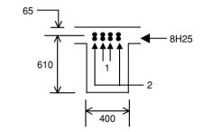
Note that, in practice, it would be difficult to hold bars 1 in place and a spacer bar would be needed between the two layers of reinforcement. This would reduce the value of the effective depth, but this aspect has been ignored in the calculations.
