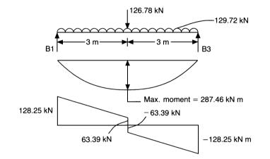
Hence, the design moment for beam B1–B3 is 287.46 kN m and occurs at mid-span and the design shear force is 128.25 kN and occurs at the supports.
