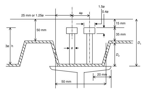
Fig. 4.45 Geometrical requirements for placing of studs (CIRIA Report 99).
