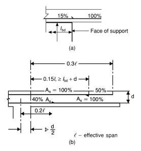
Fig. 8.26 Simplified curtailment rules for slabs (a) simple support (b) continuous member.
