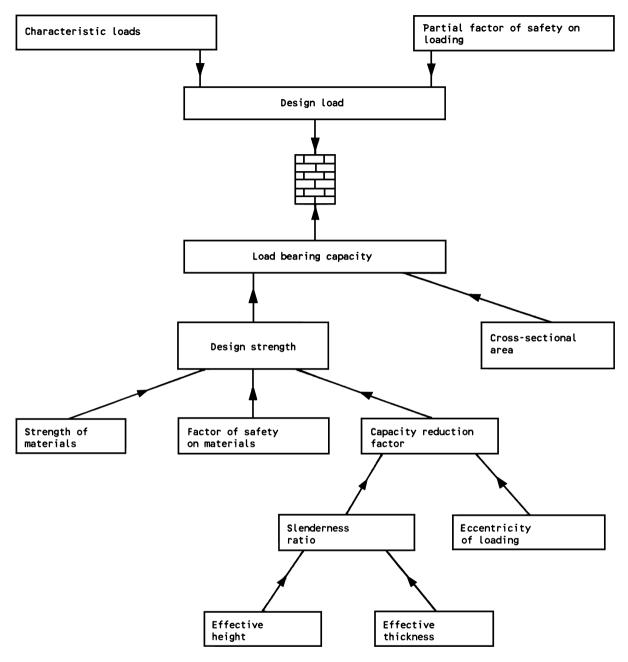
Fig. 5.16 Design procedure for vertically loaded walls.
