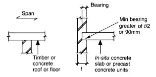
Fig. 5.11 Details of horizontal supports providing enhanced resistance.
