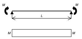
Fig. 4.21 Standard case for buckling.
