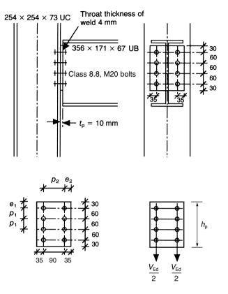
CHECK POSITIONING OF HOLES FOR BOLTS
