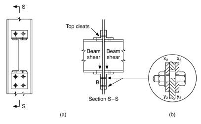
Fig. 4.53 Double shear failure.
