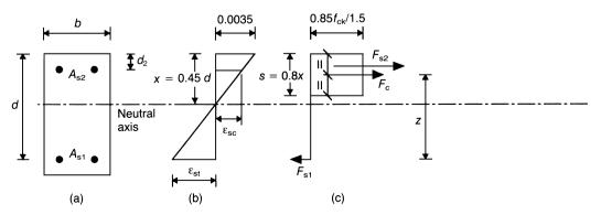
Fig. 8.8 Doubly reinforced section (a) Section (b) Strains (c) Stress Block (EC 2).
