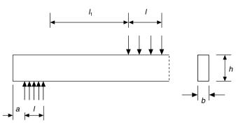
Fig. 11.5 Member on discrete support (based on Fig. 6.2b, prEN 1995-1-1: A1: 2007).
