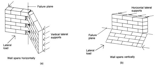
Fig. 5.22 Failure modes of walls subject to lateral loading: (a) failure perpendicular to bed joint; (b) failure parallel to bed joint.
