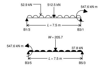
Taking moments about end B3/1 of beam B1/3, the reaction at end B1/3,  $R_{B1/3}$ , is
