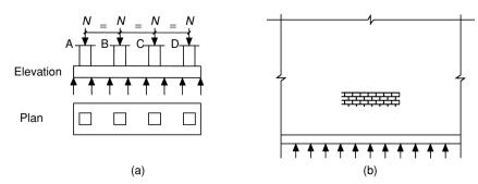
Fig. 3.71 Strip footings: (a) footing supporting columns; (b) footing supporting wall.
