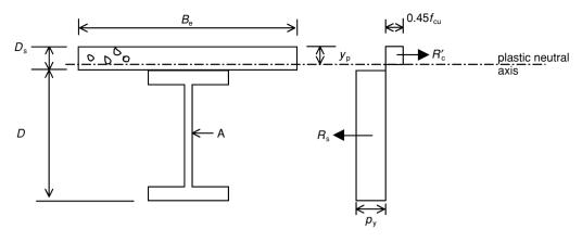
Fig. 4.41 Stress distribution when plastic neutral axis lies within concrete flange.
