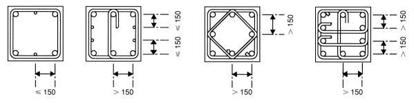
Fig. 3.103 Arrangement of links in columns.
