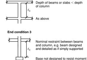
Fig. 3.90 Column end restraint conditions.
