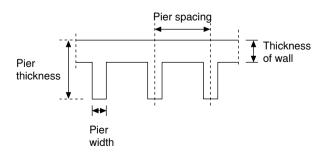
Fig. 10.2 Diagrammatic view of the definitions used in Table 10.6 (Fig. 5.2, EC 6).
