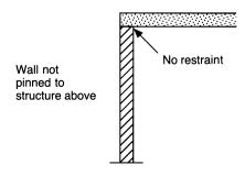
Fig. 5.23 Detail providing free edge.
