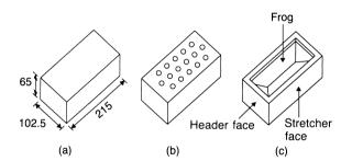
**Fig. 5.5** Types of bricks: (a) solid; (b) perforated; (c) frogged.
