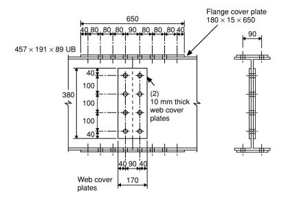
Assume that (1) flange cover plates resist the design bending moment, M and (2) web cover plates resist the design shear force, F, and the torsional moment (= Fe), where e is half the distance between the centroids of the bolt groups either side of the joint.
