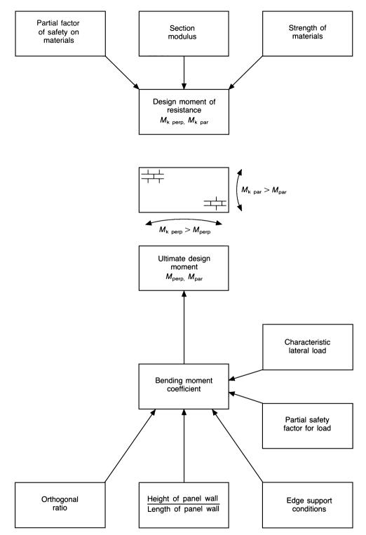
Figure 5.27 Design procedure for laterally loaded panel walls.
