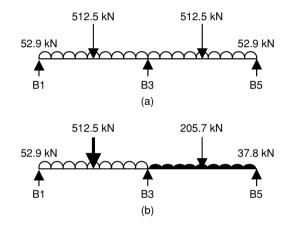
Fig. 3.45 Load cases: (a) load case 1 (b) load case 2.
