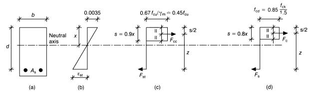
Fig. 8.7 Singly reinforced section with rectangular stress block (a) Section (b) Strains (c) Stress Block (BS 8110) (d) Stress Block (EC 2)
