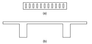
Fig. 3.56 Precast concrete floor units: (a) hollow core plank (b) double 'T' unit.
