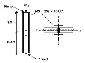
RESISTANCE OF CROSS-SECTION – COMPRESSION Design resistance of section for uniform compression,  $N_{c,Rd} = 2084.5$  kN, as above.
