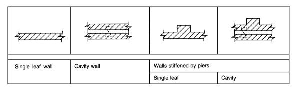
Fig. 5.8 Masonry walls.
