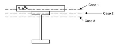
Fig. 4.40 Plastic neutral axis positions.
