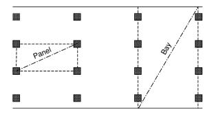
Fig. 3.62 Definition of panels and bays (Fig. 3.7, BS 8110).
