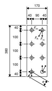
Thus bearing capacity of single web plate = 104.7 kN and bearing capacity of two web plates =  $2 \times 104.7 = 209$  kN >  $F_{R}$ . Hence web cover plates are adequate in bearing.
