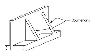
Fig. 3.79 Counterfort retaining wall.
