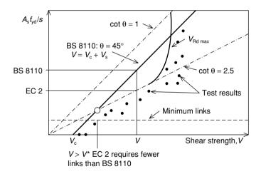
Fig. 8.10 Influence of links on shear strength.
