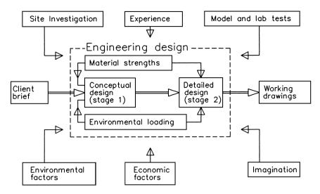
Fig. 1.1 Inputs into the design process.
