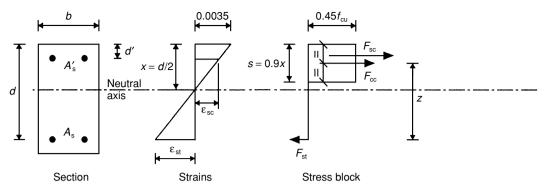
Fig. 3.33 Section with compression reinforcement.
