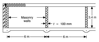
(b) A 102.5 mm brick wall is to be designed to withstand a wind pressure of 550 N m<sup>-2</sup>. For the support conditions shown in (i) and (ii) below, determine suitable brick/mortar combinations for the two cases. Assume the masonry units are category II and the category of construction control is normal.
