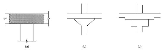
Fig. 3.53 Methods of reducing shear stresses in flat slab construction: (a) deep slab and large column; (b) slab with flared column head; (c) slab with drop panel and column head.
