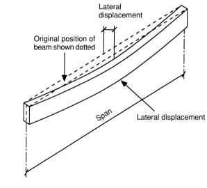
Fig. 6.5 Lateral buckling.
