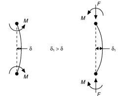
Fig. 6.8 Bending in timber columns.
