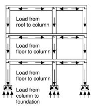
Foundation loads resisted by ground
