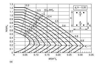
Fig. 8.32 Typical column design charts for use with EC 2.
