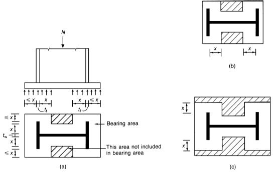
Fig. 9.7 Area in compression under base plate: (a) general case; (b) short projection; (c) large projetion (Fig. L. 1, ENV EC3).
