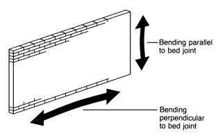
Fig. 5.21 Panel wall subject to two-way bending.
