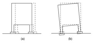
Fig. 3.69 Foundation failures: (a) sliding failure; (b) overturning failure.
