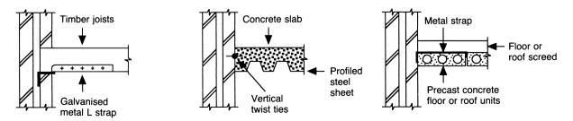
Fig. 5.10 Details of horizontal supports providing simple resistance.
