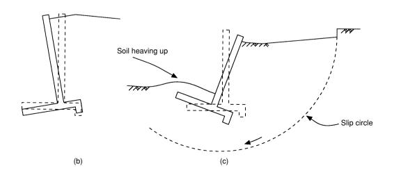
Fig. 3.81 Modes of failure: (a) sliding; (b) overturning; (c) slip circle.
