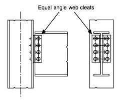
Fig. 9.13 Typical bolted double angle web cleat beam-tocolumn connection.
