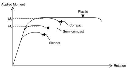
Fig. 4.10 Typical moment/rotation characteristics of different classes of section.
