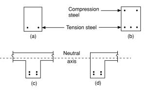
Fig. 3.12 Beam sections: (a) singly reinforced; (b) doubly reinforced; (c) T-section; (d) L-section.
