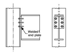
Fig. 9.11 Typical bolted beam-to-column connection.
