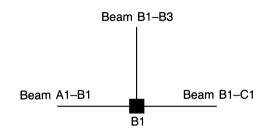
Column B1 supports the reactions from beams A1–B1, B1–C1 and B1–B3 and its self-weight. From the above, the reaction at B1 due to beam B1–C1 is 64.86 kN and from beam B1–B3 is 128.25 kN. Beam A1–B1 supports only its self-weight =  $0.98 \times 3 = 2.94$  kN. Hence reaction at B1 due to A1–B1 is 2.94/2 = 1.47 kN. Since the column height is 3 m, self-weight of column =  $0.84 \times 3 = 2.52$  kN. Hence
