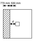
Ultimate shear force (V) = load on shaded area =  $p_s \times area = 217(3 \times 0.770) = 501$  kN Design shear stress, v, is
