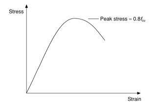
Fig. 3.6 Actual stress-strain curve for concrete in compression.
