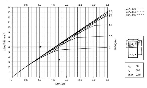
Fig. 3.35 Design chart for doubly reinforced beams (based on chart 7, BS 8110: Part 3).
