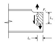
Fig. 4.56 Block shear. (Based on Fig. 22, BS 5950)
