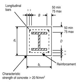
Reinforcement: steel fabric type D98 (BS 4483) or  $\ge$  5 mm diameter longitudinal bars and links at a maximum spacing of 200 mm
