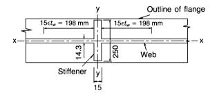
When checking the buckling resistance, the effective cross-section of a stiffener should be taken as including a width of web plate equal to  $30\varepsilon t_w$ , arranged with  $15\varepsilon t_w = 15 \times (235/275)^{0.5}14.3 = 198$  mm each side of the stiffener. Buckling length,  $l \ge 0.75 h_w = 0.75 \times 718.8 = 539$  mm Radius of gyration of stiffened section,  $i_{xy}$  is
