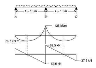
The results can be used to obtain moment and reaction coefficients by expressing in terms of W and L, where W is the load on one span only, i.e. 100 kN and L is the length of one span, i.e. 10 m, as shown in *Fig. 3.38*. The coefficients enable the bending moments and shear forces of any two equal span continuous beam, subjected to uniformly distributed loading, to be rapidly assessed.
