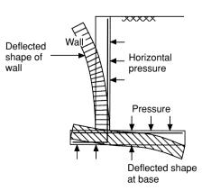
Fig. 3.2 Cantilever retaining wall.
