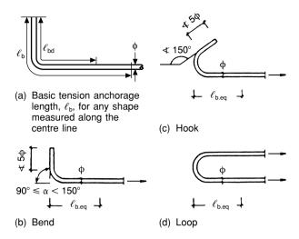
Fig. 8.18 Common methods of anchorage. Equivalent anchorage lengths for bends, hooks and loops (based on Fig. 8.1, EC 2)
