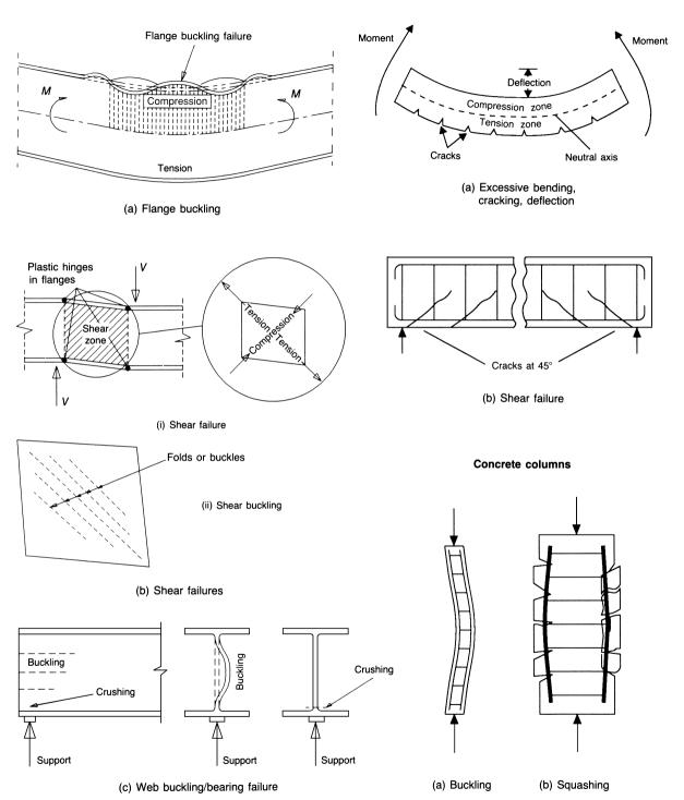
Fig. 1.3 Typical modes of failure for beams and columns.
