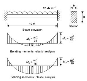
Fig. A.2 Beam with built-in supports.
