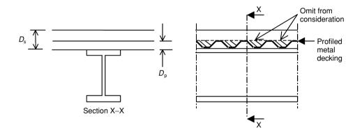
Fig. 4.43 Slab thickness and depth of metal decking.
