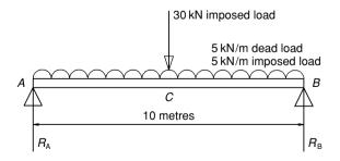
Fig. 4.11 Loading for example 4.1.
