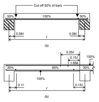
Fig. 3.27 Simplified rules for curtailment of bars in beams: (a) simply supported ends; (b) continuous beam.
