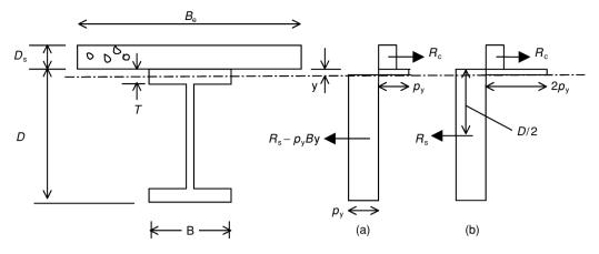
Fig. 4.42 Stress distribution when plastic neutral axis lies within steel flange.
