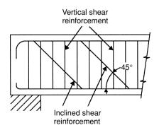
Beam with vertical and inclined shear reinforcement.
