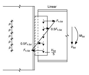
Fig. 9.14 Distribution of loads between fasteners (Fig. 6.5.7, ENV EC 3).
