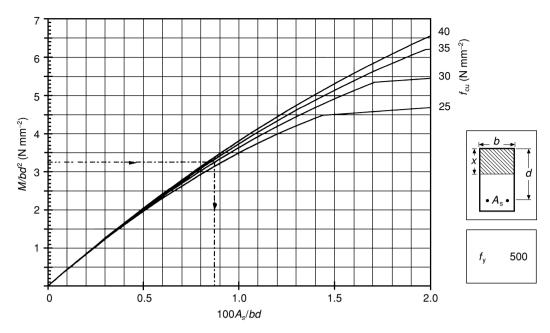
Fig. 3.20 Design chart for singly reinforced beam (based on chart No. 2, BS 8110: Part 3).
