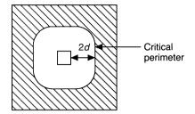
Check punching shear at 2d from face of column. Basic control perimeter,  $u_1$ , is
