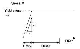
Fig. 2.6 Stress-strain plot for steel.
