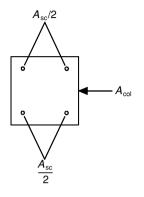
Since the column is axially loaded use equation 3.40
