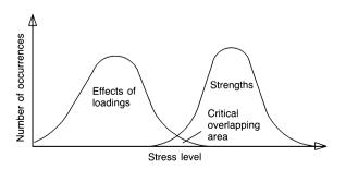
Fig. 1.2 Relationship between stress and strength.
