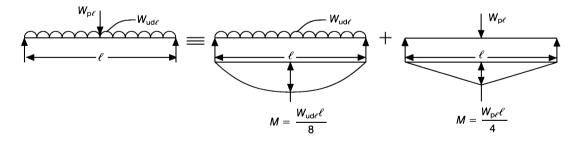
By inspection, the maximum bending moment and shear force for both load cases occur at beam mid-span and supports respectively. Thus, the design moment, M, is given by
