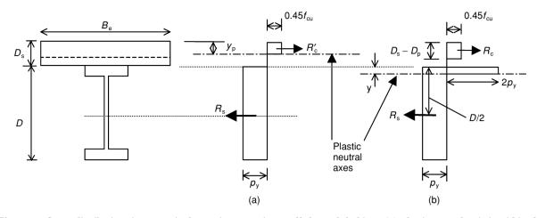
Fig. 4.44 Stress distributions in composite beams incorporating profiled metal decking: (a) plastic neutral axis is within the concrete flange (b) plastic neutral axis is within the steel flange.
