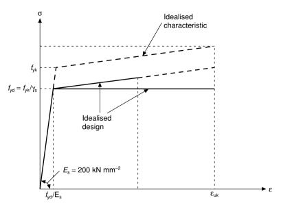
Fig. 8.5 Design stress strain diagram for steel reinforcement (Fig 3.8, EC 2).
