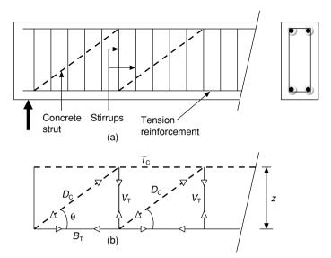
Fig. 8.9 (a) Beam and reinforcement (b) analogous truss.
