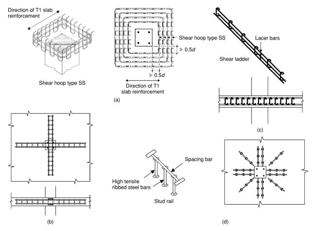
Fig. 3.54 Prefabricated punching shear reinforcement for flat slabs: (a) shear hoops (b) ACI shear stirrups (c) shear ladders (d) stud rails. Typical arrangements for an internal column.
