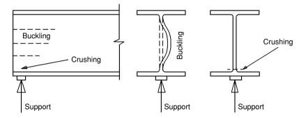
Fig. 4.7 Web buckling and web bearing failures.
