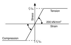
Fig. 3.9 Design stress-strain curve for reinforcement (Fig. 2.2, BS 8110).
