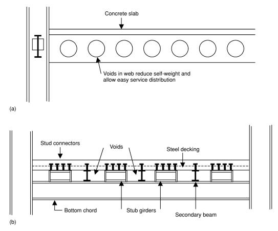
Fig. 4.37 Long span structures: (a) cellular beams (b) stub-girder.
