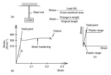
Fig. 4.1 Stress-strain curves for structural steel: (a) schematic arrangements of test; (b) actual stress-strain curain curve from experiment; (c) idealised stress-strain relationship.
