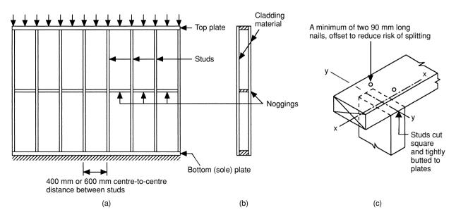
Fig. 6.9 Details of a typical stud wall: (a) elevation; (b) section; (c) typical fixing of top and bottom plates to studs.
