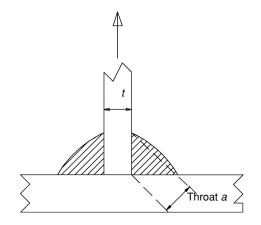
Fig. 4.58 Special fillet weld.
