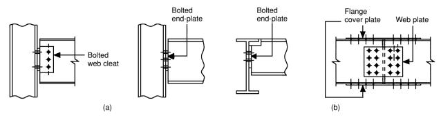
Fig. 4.50 Typical connections: (a) beam to column; (b) beam to beam.
