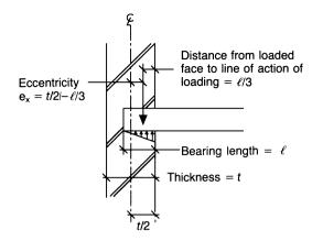
Fig. 5.14 Eccentricity for wall supporting single floor.
