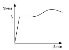
Fig. 3.8 Actual stress-strain curve for reinforcement.
