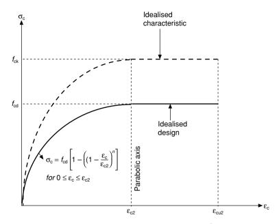
Fig. 8.3 Parabolic-rectangular stress-strain diagram for concrete ( $f_{ck} \leq 50 N mm^{-2}$ ) in compression (Fig. 3.3, EC 2).
