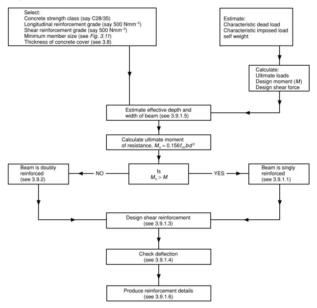
Fig. 3.48 Beam design procedure.
