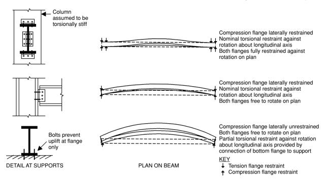
Fig. 4.20 Restraint conditions.
