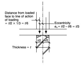
Fig. 5.15 Eccentricity for wall supporting continuous floor.
