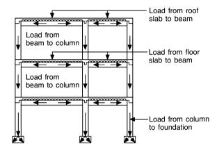
Fig. 2.1 Sequence of load transfer between elements of a structure.
