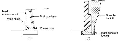
Fig. 3.77 Gravity retaining walls: (a) mass concrete wall; (b) masonry wall.
