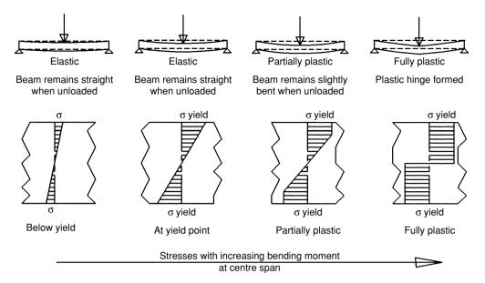
Fig. 4.4 Bending failure of a bearn.
