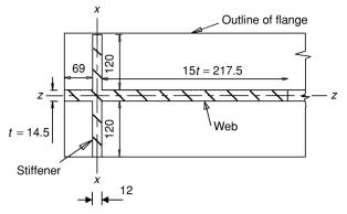
Fig. 4.18 Plan of web and stiffener.
