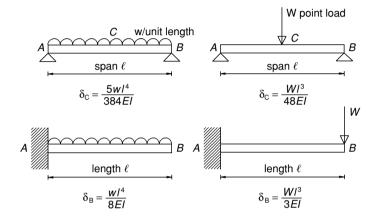
**Fig. 4.14** Deflections for standard cases. E = elastic modulus of steel (205 kN/mm<sup>2</sup>) and I = second moment of area (x-x) of section.
