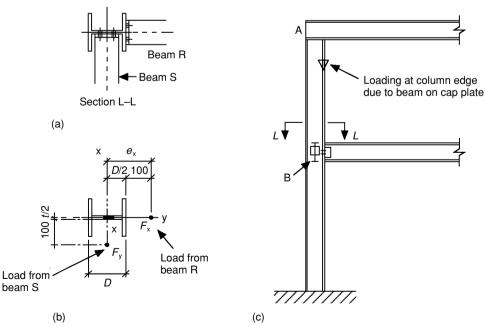
Fig. 4.27 Load eccentricity for columns in simple construction.
