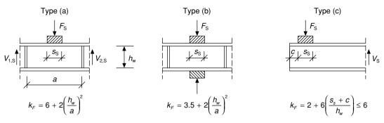
Fig. 9.3 Different types of forces applied to a web and associated buckling coefficients (Fig. 6.1, EC 3-5).
