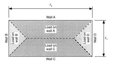
**Fig. 3.58** Plan of two-way spanning slab.  $l_x$  length of shorter side,  $l_y$  length of longer side. Provided  $l_y/l_x \le 2$  slab will span in two directions as indicated.
