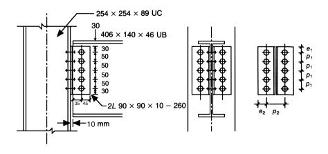
CHECK POSITIONING OF HOLES FOR BOLTS
