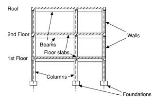
Fig. 3.1 Some elements of a structure.
