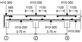
Distribution steel is H10-350 ( $A_s = 224 \text{ mm}^2/\text{m}$ )
