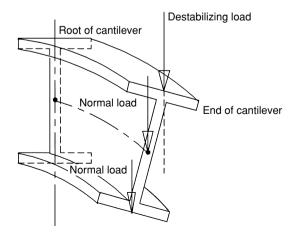
Fig. 4.8 Lateral torsional buckling of cantilever.
