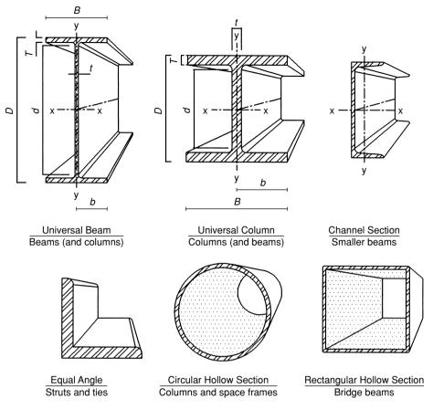
Fig. 4.2 Standard rolled steel sections.
