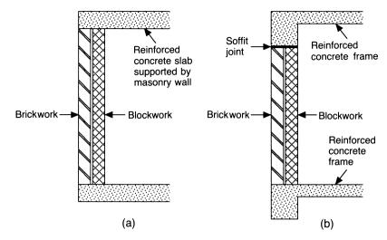
Fig. 5.2 (a) Load-bearing and (b) non-load-bearing walls.
