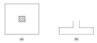
Fig. 3.70 Pad footing: (a) plan; (b) elevation.
