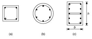
Fig. 3.84 Column cross-sections.
