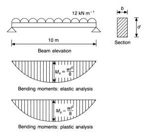
Fig. A.1 Simply supported beam.
