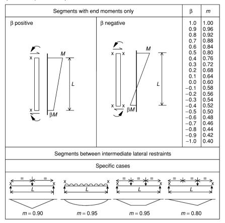
**Table 4.16** Equivalent uniform moment factor m for flexural buckling(Table 26, BS 5950)
