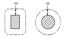
Fig. 8.29 Critical perimeters (Fig. 6.13, EC 2).
