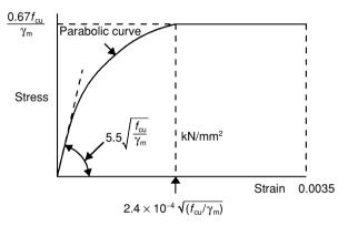
Fig. 3.7 Design stress-strain curve for concrete in compression (Fig. 2.1, BS 8110).
