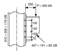
Since the bolts are subject to combined shear and tension, the bolts should be checked for shear, tension and combined shear and tension separately.
