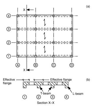
Fig. 3.36 Floor slab: (a) plan (b) cross-section.
