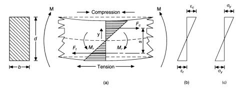
Fig. 2.7 Strain and stress in an elastic beam.
