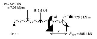
$M = 770.3 - 385.4x + \frac{7.05x^2}{2}$ . Solving for M = 651 kNm implies that the theoretical cut-off point of mark 1 bars
