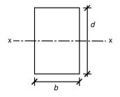
Fig. 6.4 Section modulus.
