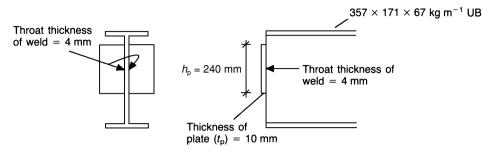
Ultimate tensile strength of S 275 steel  $(f_u) = 430 \text{ N mm}^{-2}$  (*Table 9.16*) Correlation factor  $(\beta_w) = 0.85$ Throat thickness of weld (a) = 4 mmPartial safety factor for welds  $(\gamma_{M2}) = 1.25$
