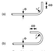
For mild steel bars minimum  $r = 2\Phi$ For high yield bars minimum  $r = 3\Phi$  or  $4\Phi$  for sizes 25 mm and above
