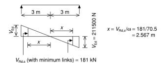
Where  $V_{Ed} < V_{Rd,cr}$  provide minimum shear reinforcement,  $\rho_{w,min}$ , according to
