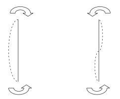
Fig. 8.31 Column buckling modes.
