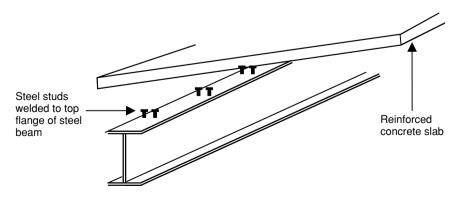
Fig. 4.34 In-situ reinforced concrete slab.
