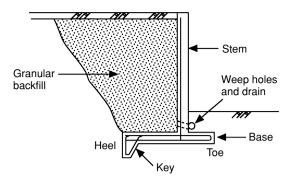
Fig. 3.78 Cantilever wall.
