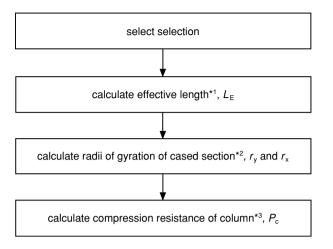
Fig. 4.31 Design procedure for axially loaded cased columns.
