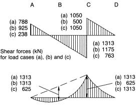
Bending moments (kN m) for load cases (a), (b) and (c)
