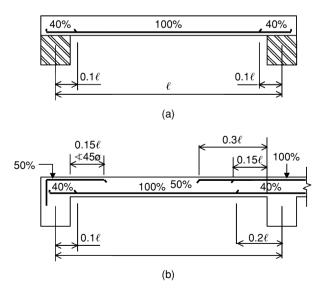
Fig. 3.60 Simplified rules for curtailment of bars in slabs: (a) simply supported ends; (b) continuous slab (based on Fig. 3.25, BS 8110).
