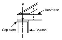
Fig. 4.28 Column supporting a roof truss.
