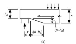
Fig. 11.3 End notched beams (Fig. 6.11, EC 5).
