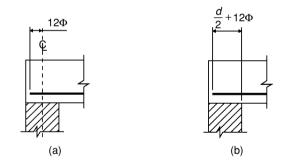
Fig. 3.28 Anchorage requirements at simple supports.
