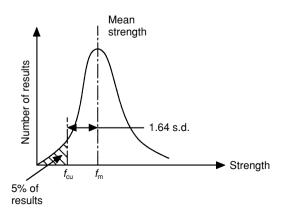
Fig. 3.3 Normal frequency distribution of strengths.
