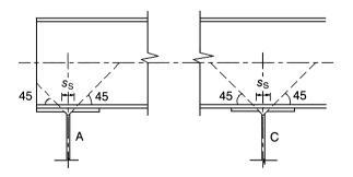
Stiff bearing length,  $s_s \approx 2t_f + t_w + r = 2 \times 36.6 + 21.5 + 24.1 = 118.8 \text{ mm}$ Since the load is applied through the flange and is resisted by shear forces in the web (i.e. load type (a) in *Fig. 9.3*),  $k_F$  is given by
