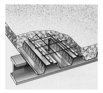
Fig. 4.35 Composite metal deck floor.
