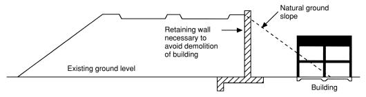
Fig. 3.76 Section through road embankment incorporating a retaining wall.
