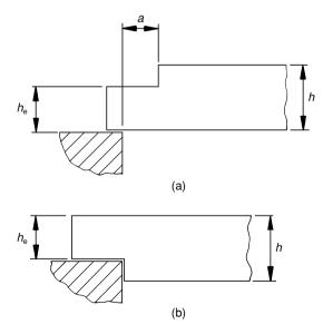
Fig. 6.2 Notched beams: (a) beam with notch on top edge; (b) beam with notch on underside (Fig. 2, BS 5268).
