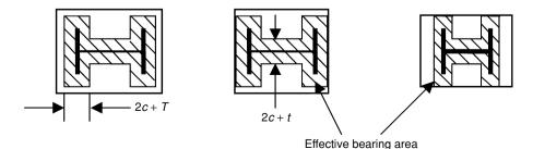
The required minimum baseplate thickness,  $t_{\rm p}$ , is given by
