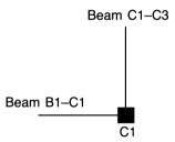
Column C1 supports the reactions from beams B1–C1 and C1–C3 and its self-weight. From the above, the reaction at C1 due to beam B1–C1 is 64.86 kN. Beam C1–C3 supports the reactions from B2–C2 (= 126.78 kN) and its self-weight (=  $0.98 \times 6$ ) = 5.88 kN. Hence the reaction at C1 is (126.78 + 5.88)/2 = 66.33 kN. Since the column height is 3 m, self-weight =  $0.84 \times 3 = 2.52$  kN. Hence
