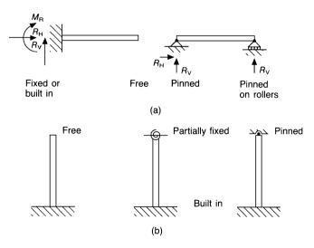
Fig. 2.5 Typical beams and column support conditions.
