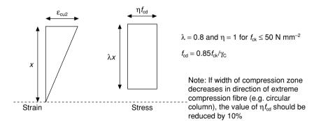
Fig. 8.4 Simplified stress block for concrete at the ultimate limit state (based on Fig. 3.5, EC 2).
