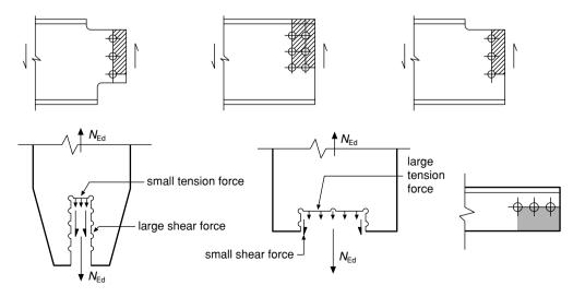
Fig. 9.12 Block tearing – net tension and shear areas (Fig. 3.8, EC 3-8).
