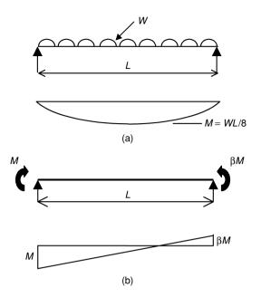
Fig. 4.22 Load cases less susceptible to buckling.
