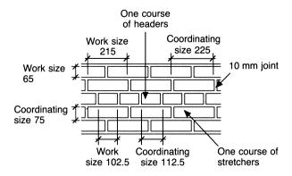
Fig. 5.6 Coordinating and work size of bricks.
