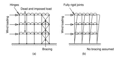
Fig. 4.3 (a) Simple and (b) continuous design.
