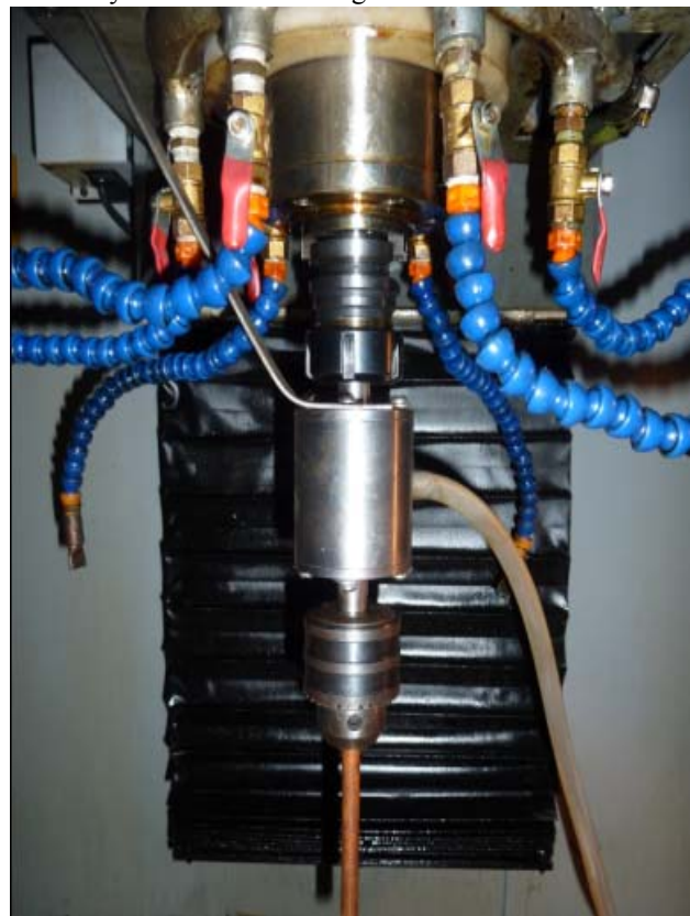
Fig 5. Photograph of the rotary joint structure.
