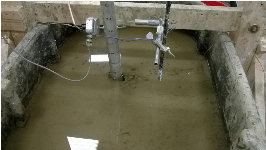
Figure 5.18: Creation of a gap behind the 2-inch diameter pile during monotonic load test, normally consolidated Gulf of Mexico clay bed
