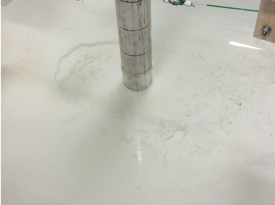
Figure 3.43: Disturbed Soil around 3" Diameter Monopile after Cyclic Tests
