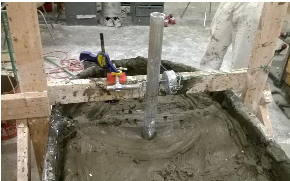
Figure 3.17: Heavily overconsolidated Gulf of Mexico clay bed with a 2-inch diameter pile installed and ready to be tested
