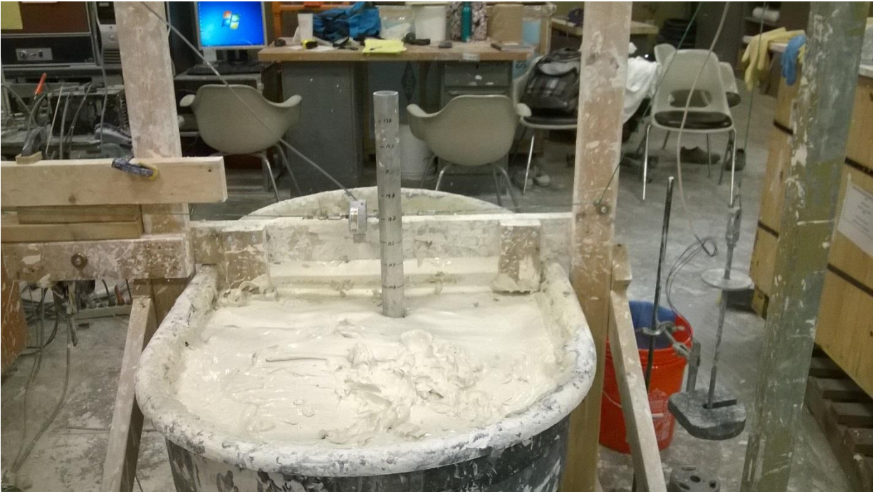
Figure 3.59: 2-inch diameter monopile during cyclic test, overconsolidated soil bed
