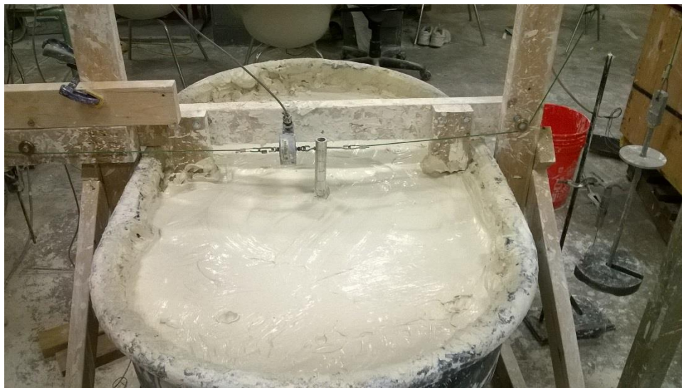
Figure 3.9: 100-gallon Rubbermaid stock tank which contained the soil bed with the heavily overconsolidated kaolinite clay (1-inch diameter pile installed is also shown)
