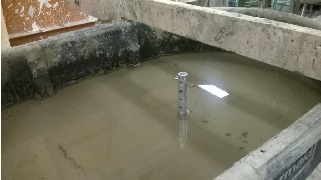
Figure 3.23: Normally consolidated GoM clay bed with 1-inch diameter pile installed and ready to be tested
