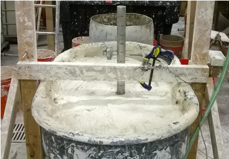
Figure 3.13: Heavily overconsolidated kaolinite clay bed with a stiff crust with 2-inch diameter pile installed and ready to be tested
