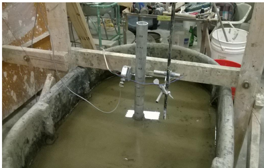
Figure 3.62: Normally consolidated GoM clay bed with 2-inch diameter pile installed and ready to be tested
