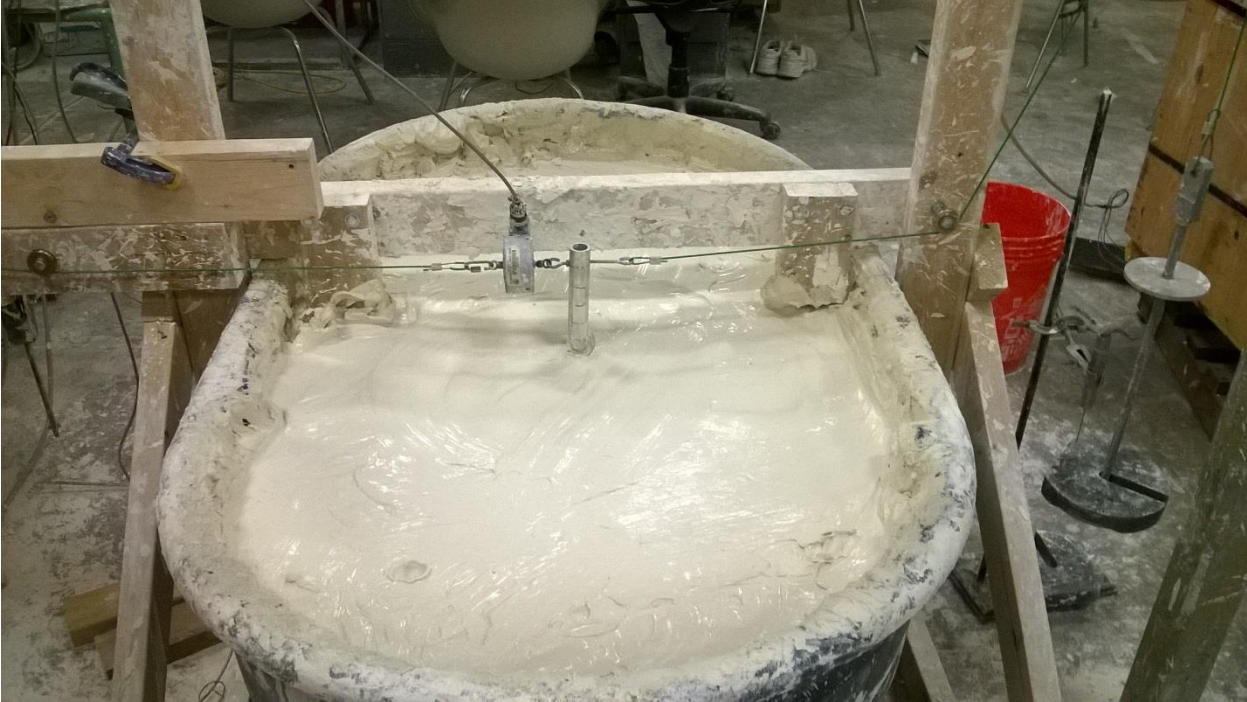
Figure 3.58: 1-inch diameter monopile during cyclic test, overconsolidated soil bed
