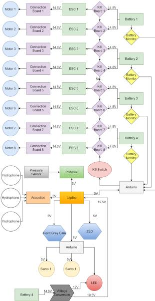
Fig. 5: Electrical Wiring Diagram
